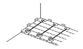
3. Lay one row of plank along the entire length of the working line.
