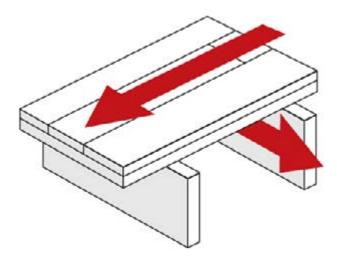
Check with the joist or truss Manufacturer to determine if cross-bracing is allowed with that system. Should it not be compatible with the joist or truss Manufacturer, sheeting the sub floor with a second layer of CD or better grade plywood would then be the only option. (See double layer sub floors section).
