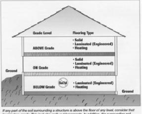
If any part of the soil surrounding a structure is above the floor of any level, consider that level below-grade. This includes waik-out basements. In addition, the surrounding soil should be sloped away from the structure with at least 6 inches of fail over the first 10 feet.
